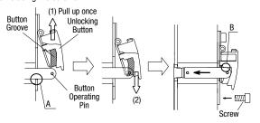
After fastening the screws, check if locking and unlocking operations can be performed.
