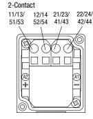
When connecting the NC contact (11-12, 21-22) of door monitor circuit and NC contacts (41-42, 51-52) of the lock monitor circuit in a series as an input to a safety circuit, connect 12-41 or 22-51.
