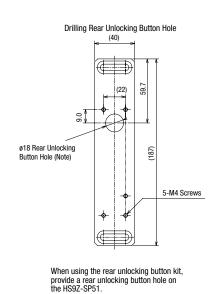
Note: With the mounting hole dimension, the rear unlocking button rod does not touch the mounting hole even when the interlock switch moves sideways.
