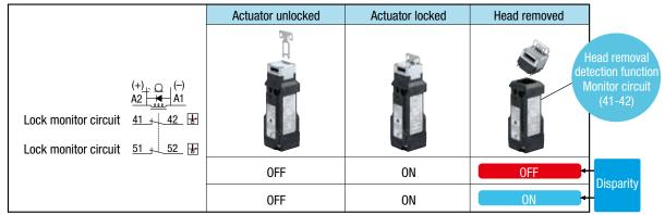
Note: Head removal detection function is not a direct opening action mechanism.
